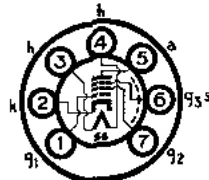
The BRIMAR 6065 is an indirectly heated vari-mu R.F. pentode, suitable for use as an R.F. or I.F. amplifier, and in a variety of applications where vari-mu characteristics are required.
